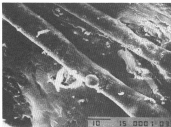
Figure 1. SEM photograph showing the bands observed in an as-grown needle crystal. Bands are formed due to temperature oscillations within the melt. See text for discussion.
